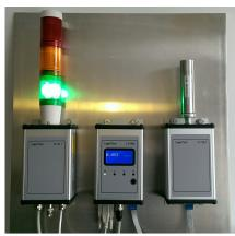
The devices has 5 relay outputs that work synchronized with the front panel LEDs and the buzzer enabling the execution of alarm, fail and controlling order towards the connected systems.
