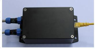
Modbus-TCPserver, which serves datas from its RAM to its connected clients. The listen-only mode is suitable for parallel operation with the existing SCADA/DAQ system without disturbing it.
